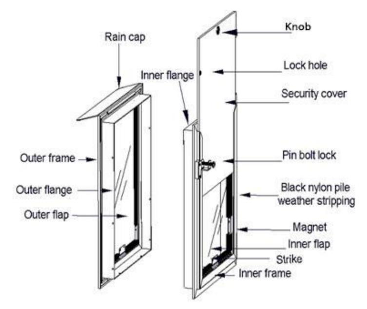
The Hale Pet Door™ "Door Model" is a popular model. It's self-framing and self-supporting design makes it easy to install in almost any door location. No need to frame out the door. Just cut the correct size rough opening in the door, slip the inside and outside frames together and attach with provided screws. Instructions for installation included in the box or on our website. We offer technical support when needed and professional installation is available in many locations nationwide.
