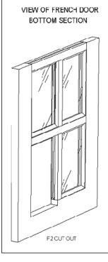
Step 5: First, find the removable molding that is holding the glass in the French door. (IF THE FRENCH DOOR DOESN'T HAVE **REMOVABLE** MOLDING, **PLEASE CALL TECHNICAL SUPPORT** FOR HELP). Removable molding can usually be identified by staples or nail heads. If the molding has been painted over or you can't find staples or nails, try sliding a putty knife under the molding.
