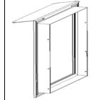
**Step 9:** Using the pre-drilled pilot holes in the pet door frame and the supplied drill bit, drill one hole through the inside edge of the outside frame at the bottom. Insert and loosely tighten one screw to hold it in place. Make sure the door is level and adjust if needed. Measure carefully and cut the molding to fit. Put molding around the acrylic to hold it in place. When nailing the molding back into the door, place paper or cardboard over the acrylic to protect it from the hammer.
