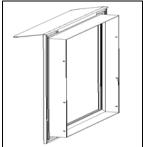
**Step 10:** Using the pre-drilled pilot holes in the pet door frame and the supplied drill bit, drill one hole into the French door with the supplied
