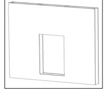
**Step 13:** Place the inside frame with attached tunnel through the wall cutout. From the outside, reach through the opening and hold the inside frame tight against the wall. Mark the tunnel with a pencil along the outside wall on all sides as shown.
