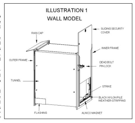
**Strikes:** Made of ferrous stainless steel. 1 1/2" long, 3/4" tall and 1/32" thick. U shaped with interior prongs, when pressed onto the vinyl flap, the barbed prongs hold firmly.
