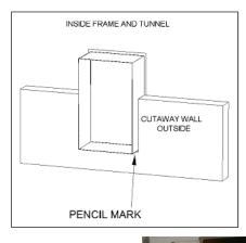
**Step 14**: Remove the interior pet door frame and tunnel from the hole. Carefully cut the tunnel along the pencil mark with metal snips to make the tunnel the correct depth for your wall. Be cautious when cutting metal so you don't accidentally cut yourself on the removed piece. Discard the metal strip that you have cut off the tunnel.
