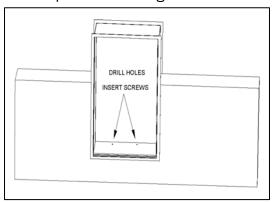
Drill holes into sides and bottom of tunnel and secure with screws. Number of holes will vary depending on the size of the pet door ordered ing
