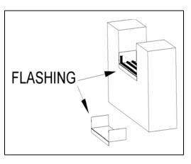
Step 16: Place the flashing into the bottom of the wall opening. The flashing should have the two side flanges pointing upward and the outside flange downward and against the outside wall as shown.
