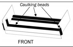
Step 15: The "Flashing" is a thin piece of aluminum with three flanges designed to aid with water containment and diversion. Caulk the flashing with latex caulking as follows: Apply two large beads on the bottom approximately 1/2" from
