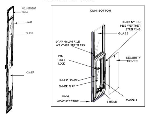
**Step 5:** Determine with the customer on which side of their patio door they want to install the Omni Panel. The stationary side is preferred, but the sliding side is slightly easier.
