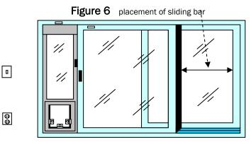
1. Choose an area approximately midway between the top and bottom of the Hale Omni Panel™ Insert. Clean the area inside the door channel and the back of the sliding door. Make sure the areas are dry. Measure from the bottom of the sliding door track and place a pencil mark in the vertical door channel. Repeat this step and mark the
