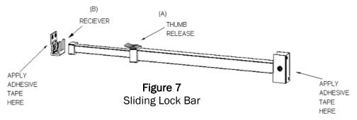
channel. (Figure 7) Peel the paper off the back of the receiver and press it very firmly onto the back of the sliding door.
