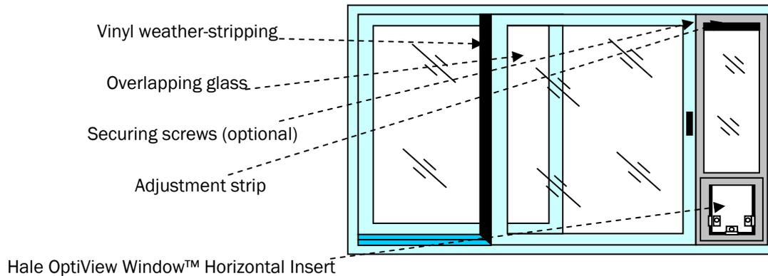
**Step 12:** If you so desire, you can put a screw or two through the window frame to prevent the window from being opened. **Be very careful that you don't drill into glass!** If you hit the window pane with either the tip of the drill bit or a screw, it will shatter. The glass in the pet door comes all the way to the edge of the frame, so don't try to drill into the pet door frame at all.
