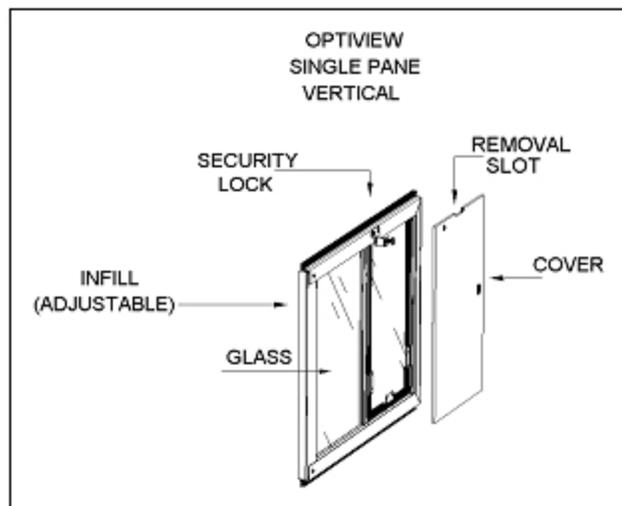
**Security Cover:** 3/16" thick GE Lexan® polycarbonate sheet. Extremely shock and impact resistant. Has a 3/8" diameter locking hole and a 3/4" diameter handle hole.
